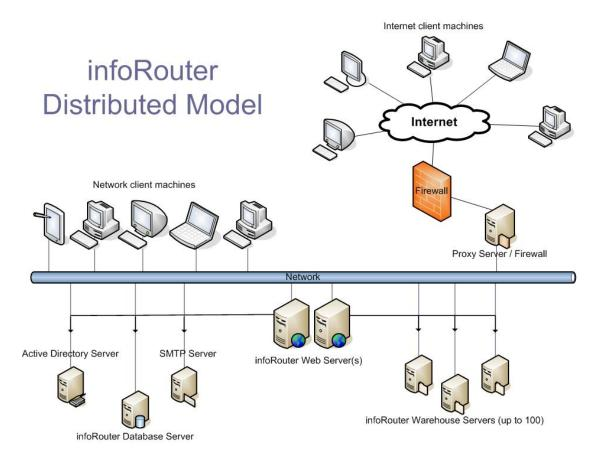
In this model, the infoRouter IIS application is on two servers, the warehouse is spread across multiple servers for load balancing and the DBMS is on its own server.
