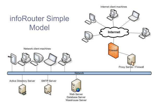
In this model, the infoRouter IIS application, the warehouse and the DBMS are all on one server.
